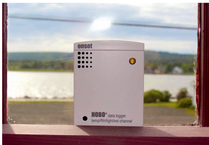
Digital data logger measures temperature and relative humidity and can be accessed by your mobile device and computer
