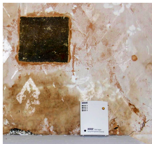
Digital data logger measures temperature and relative humidity and can be accessed by your mobile device and computer
